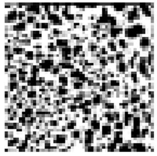
Fig. 2. A low-resolution image of the structure shown in Fig. 1 (300  $\mu$ m pixel size). The range of grey levels present in the image is due to the partial volume effect.
