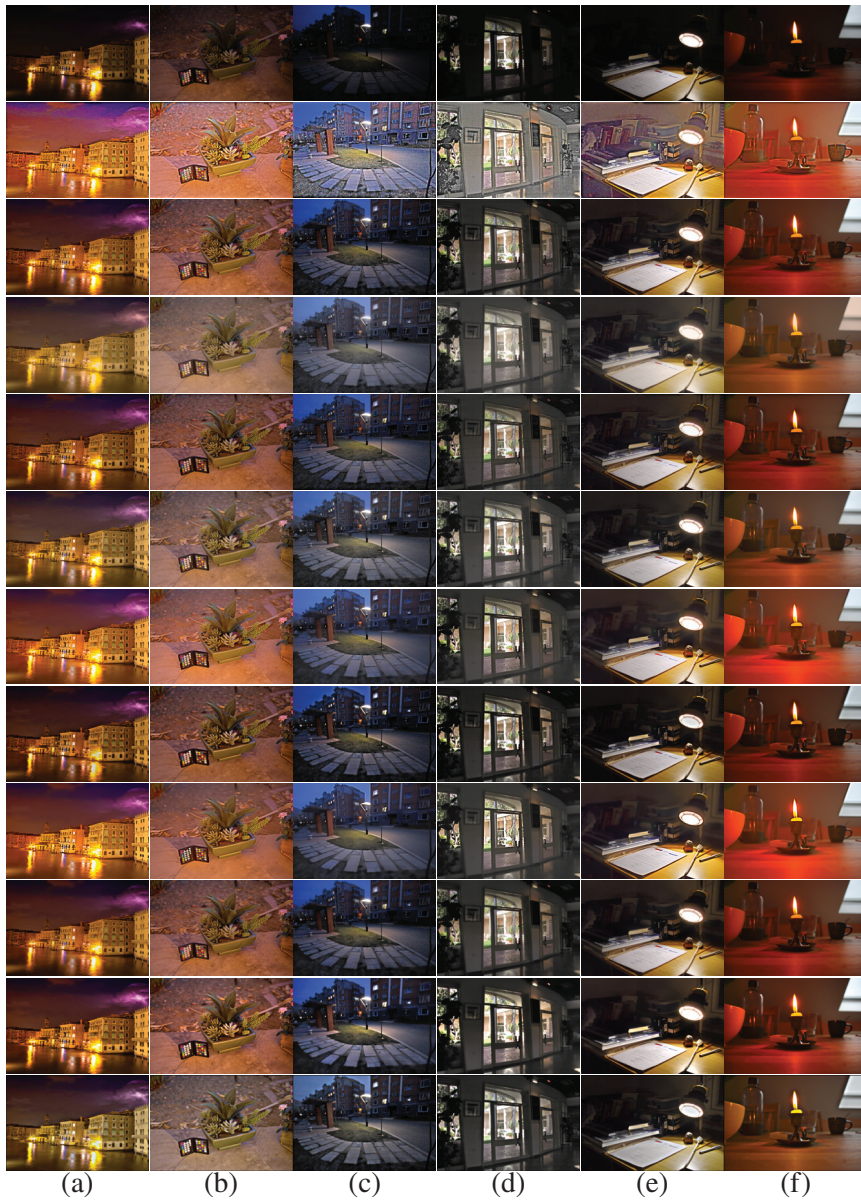
Fig. 4. Enhancement results of these algorithms on low-light images. (a) #1; (b) #3; (c) #10; (d) #BelgiumHouse; (e) #Cadik; (f) #Candle. *From top to bottom, each row denotes low-light images, LIME, STAR, RBMP, WVM, BIMEF, RRM, BRAIN, FSTAR, LR3M, SDD and the proposed algorithm, respectively.
