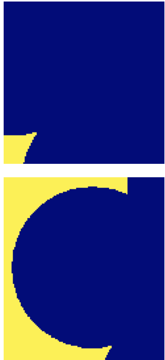
Fig. 8. We have sub-images of a pore and a pore intersection on the top and bottom pictures, respectively. The white pixel density of the top side is much higher than the white pixel density of a pore intersection, motivating the parametrization of pixel density.
