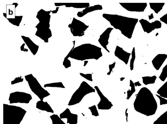
Fig. 1. Representative images from the Cu dataset: (a) RLM image and (b) corresponding binary reference mask. Ore grains are shown in black and embedding resin in white. Data reproduced from Gomes et al. (2021a).
