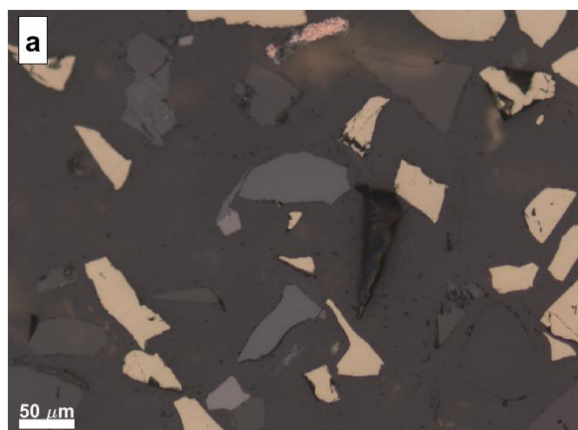
Fig. 1. Representative images from the Cu dataset: (a) RLM image and (b) corresponding binary reference mask. Ore grains are shown in black and embedding resin in white. Data reproduced from Gomes et al. (2021a).
