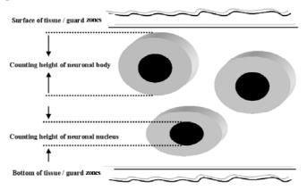
Fig. 3. Demonstrates determination of counting height (h) using either the neuronal body or neuronal nucleus in the tissue section. As illustrated, both regions of the surface and bottom of tissue are regarded as a guard zones in which neurons are not counted because of uneven tissue topography.
