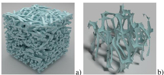
Fig. 7. Visualizations of  $512^3$  out of  $2048^3$  pixels of  $\mu$ CT-scans: (a) of a fiber fleece and (b) of a partially open foam.
