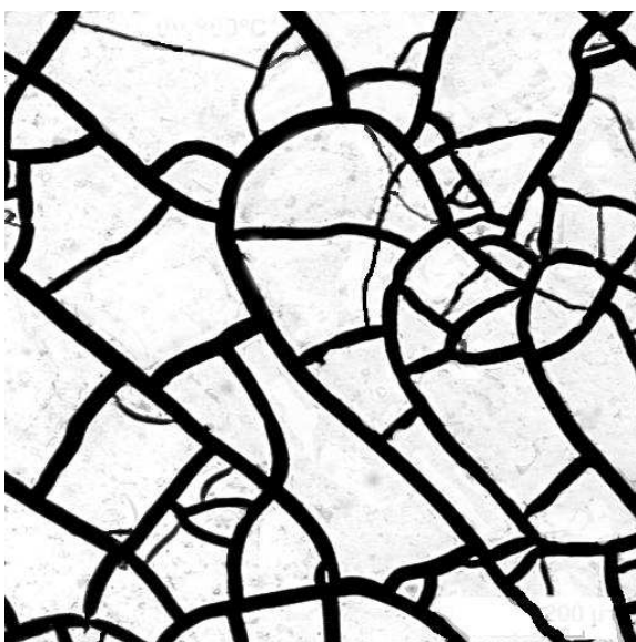
Fig. 3. Cracks in a titanium-nitride coating on cemented carbide (R. Ohser-Wiedemann).
